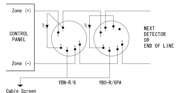
Fig 9: Connection to Conventional Control Panel
