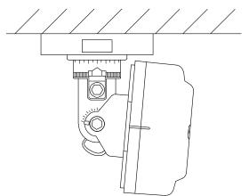
Fig 7 : Installation with ceiling bracket (YZU-A)
