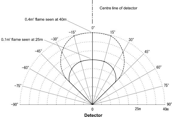
Fig 5 : Detector Field of View Plot
