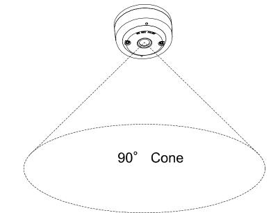
Fig 4: Conical field of view of the flame detector
