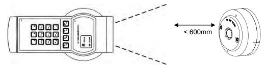
Fig 10 : Portable Flame Detector Test Unit (Model Name:016061)
