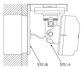
Fig 8: Installation with wall bracket (YZU-B with YZU-A)
