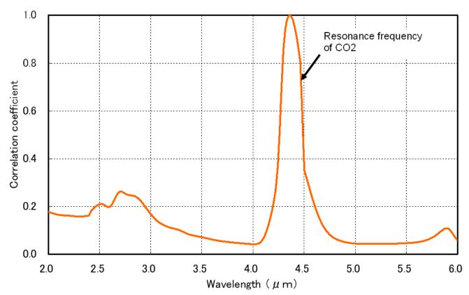
Fig 2 : Spectrum of white gas flame
