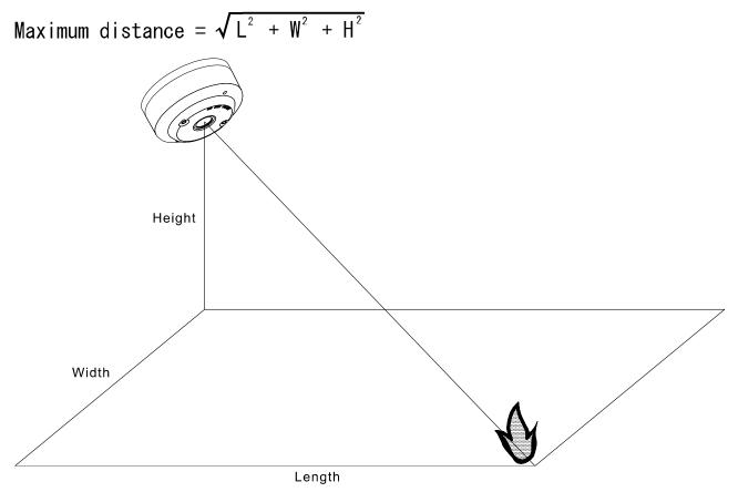
Fig 3: Calculation of distance from detector to flame
